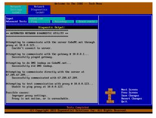
Auto test diagnosing a connection failure
